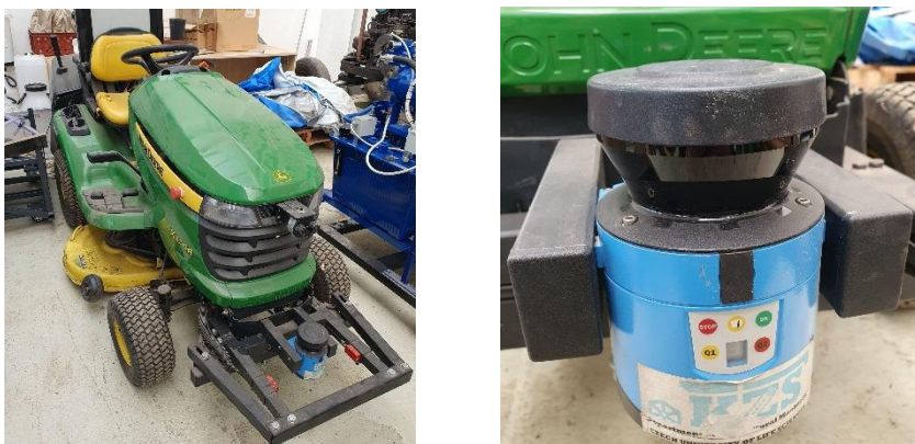
Fig. 1. a) Robot with LiDAR sensor, b) LiDAR sensor used for navigation.
