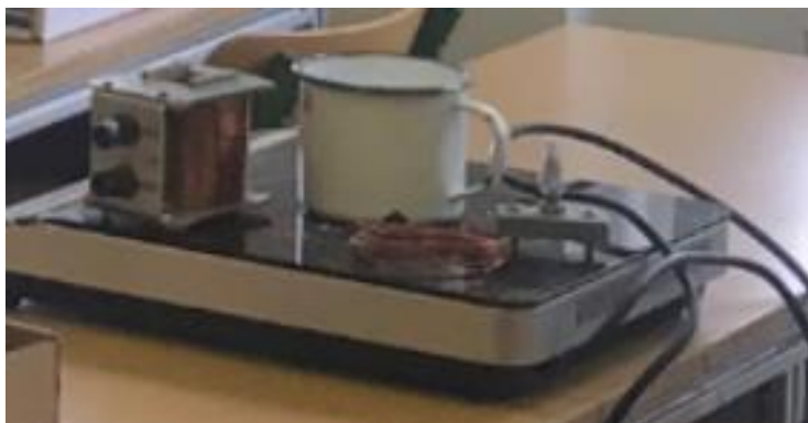
Fig. 2. Wireless charger based on an induction hob
