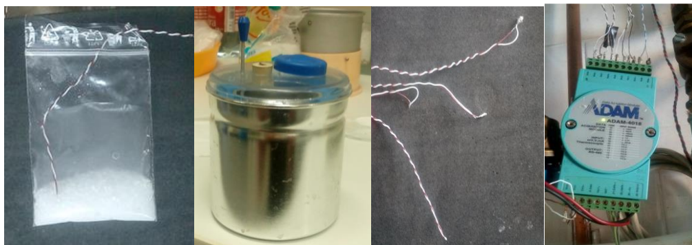
Fig. 1. Mixture sample, calorimeter, thermocouples and data logger module
