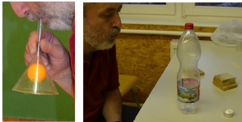
Fig. 2. Demonstration of the Bernoulli law with simple tools
