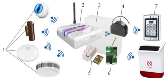
Fig. 1. The realization model: 1 – Z-Wave detectors; 2 – Fibaro HC Lite (switchboard); 3 – case; 4 – Fibaro relay FGS-211; 5 – backup power; 6 – GSM output; 7 – Z-Wave access keypad; 8 - Z-Wave alarm
